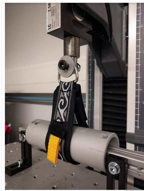
A complete wrist band closed around a cylinder as it is worn, carrying 2 500 N at the D-ring. The Velcro overlap wraps the underside of the cylinder, on the far side from the pull. Photograph: Espotel Oy tension test report, 23 April 2018.
